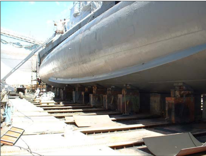
The USS Bowfin, blasted then primed with CeRam-Kote 99M
