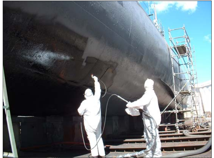
CeRam-Kote SPG applied over primer coat of CeRam-Kote 99M
